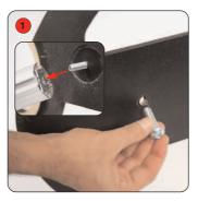
Take the base and insert a screw through the underside, through the hole, feeding it into the bottom of the LInear post.
